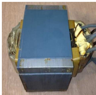
Fig. 1. Single-phase transformer with four windings.
